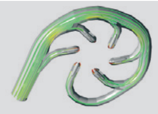
Streak lines of the optimized Gilgel Gibe II distributor line.
