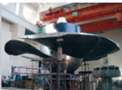
Kaplan runner for the Fuchunjiang hydro power station.
