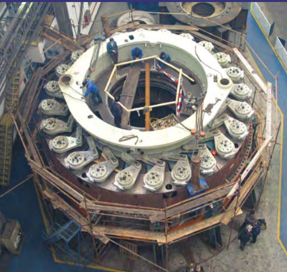
Workshop assembly of Long Tan distributor.
