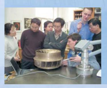
In March 2005, the model acceptance test was successfully performed at the Brunnenmühle laboratory in Heidenheim, Germany. The model turbine, designed and optimized for the unique Laxiwa power station requirements, was extensively tested. The next step will be detailed engineering and manufacture of major components for the prototype.
