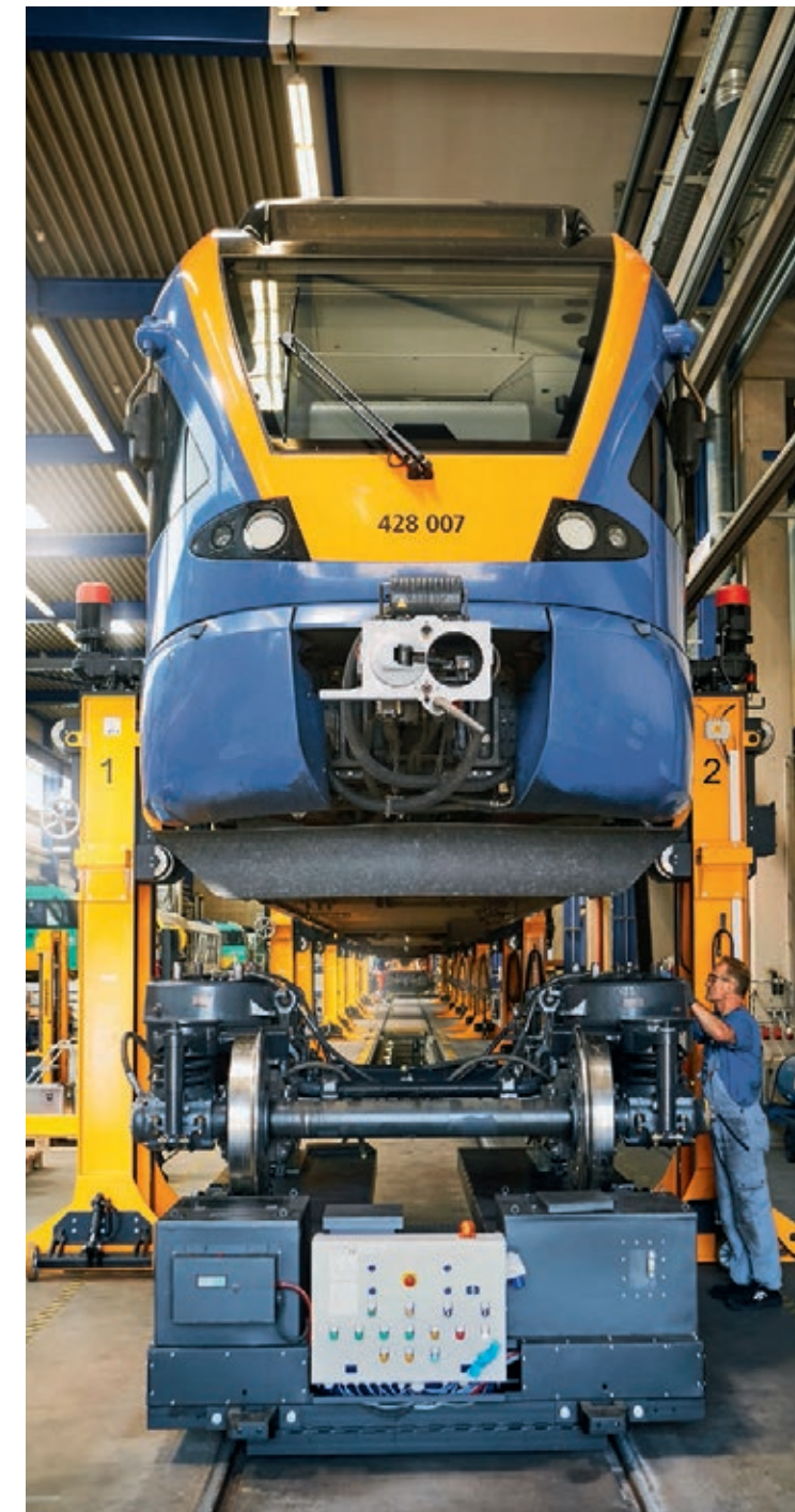
The cantus FLIRT (Fast Light Innovative Regional Train) is 74 m long and weighs 125 metric tons.
