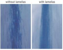
Micro-turbulence in the free jet is mainly created at the end of the nozzle by fluid friction, due to the high acceleration of the flow in this area.
