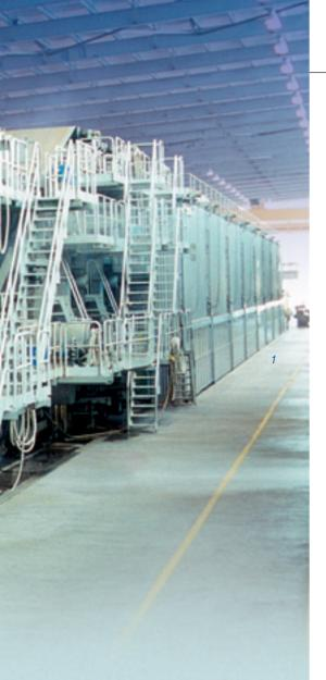
**Technical data** Wire width 5,880 mm Design speed 1,000 m/min Production 40,000 tons/year of kraft liner Basis weight 80-300 g/m<sup>2</sup> Furnish 80% kraft pulp, 20% recycled fibers
