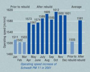
started at the end of March 2001, also after a seven-day shutdown. Only two months later, the average operating speed had increased by more than 70 m/min, and the 1,600 m/min limit exceeded with a maximum speed, so far, of 1,650 m/min.
