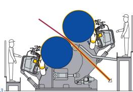
For the hard rolls ceramic coatings can also be used – **CeraSize**. These coatings are characterized by a virtually perfect constancy of shape of the surface over yearstime. Due to the high form stability of the hard roll, a longer service life of the soft mating rolls is usually also achieved.
