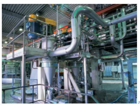
able incineration of the lightweight contaminants fraction. Rejects from the Fiberizer and drum screen are separated by a metal detector into a metal-free lightweight fraction, and a smaller heavyweight fraction containing metal. After dewatering, the lightweight fraction can, in future, be reduced by shredding to the required particle size ready for incineration.
