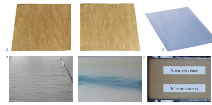
surface due to cross flows at the impingement point, induced by the macrostructures in the free jet.
