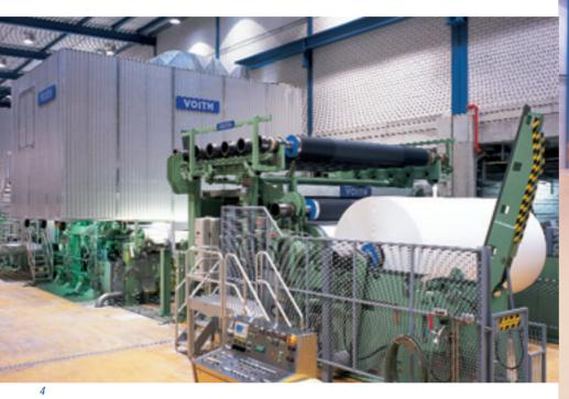
manufactured and supplied all main components – from stock preparation to paper roll transport. With today's increasingly complex production and handling, this maximal integration of all interactive process technologies under the same responsibility is proving more and more successful.
