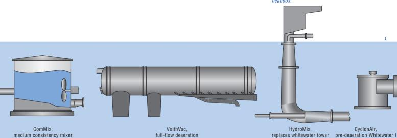
also incorporates the ComMix, HydroMix and CyclonAir components. These are specifically dimensioned and locally integrated to meet individual system requirements.
