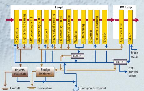
material input of about 190 t/24 h. The stock preparation included a high consistency pulper, hole screening, flotation, heavyweight contaminant cleaning, screening, lightweight cleaning, and washing. At the end of the line the stock was disperged and bleached with a reductive bleaching agent.
