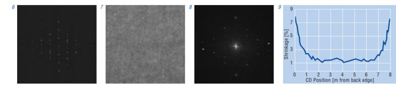
the peaks selected in *Fig. 4* are clearly also found in *Fig. 6* confirming that this forming fabric is the source of the mark in the paper, and not a press fabric as was thought by the papermaker.
