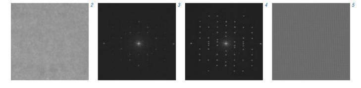
image, in which periodic elements are represented by sharp peaks and other variations by continuous shading. This is followed by interactive filtering of the FFT spectrum and an inverse FFT. This method firstly detects any periodic content in an image over a wide range of frequencies, then allows the periodic and non-periodic contributions of the image to be separated.
