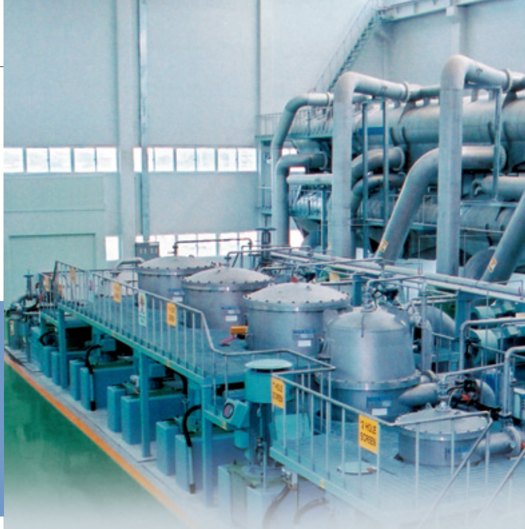
Fig. 3: Hole and slot screening (foreground) and part of the EcoCell deinking system (background).
