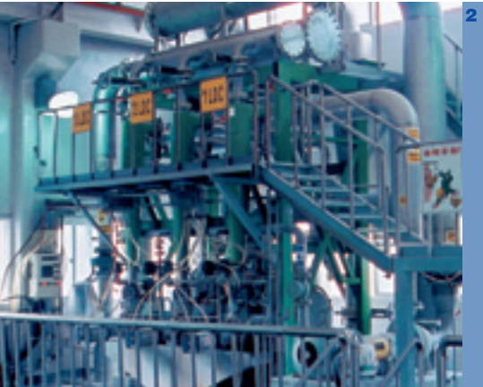
Fig. 3: Hole and slot screening (foreground) and part of the EcoCell deinking system (background).
