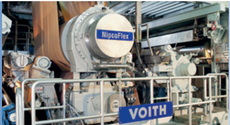
Fig. 3: Board machine 2 after the rebuild. In the foreground, the suction cylinders for filler plies with FloatLip formers.
