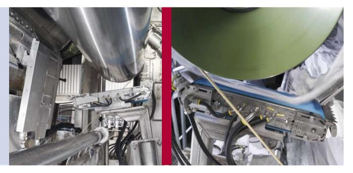
Fig. 4: Prevo threading solution on the PM in the SpeedSizer section (left: operating position; right: successful hit).
