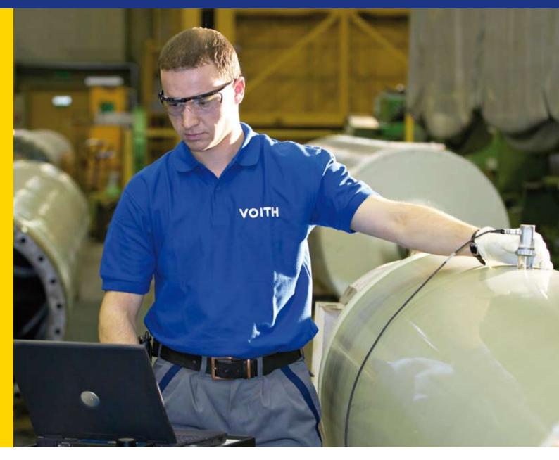
RollCare: Ultrasonic testing of a roll cover.
