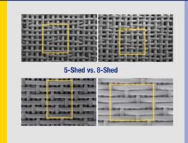
Open warp structure and sheet support mechanism.
