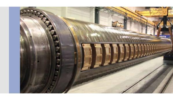
Hydrein roll in the rebuild to the Nipcorect roll.
