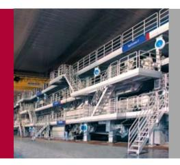
Fig. 1: On multi-ply cardboard machines, measurements can be made on the different headboxes.
