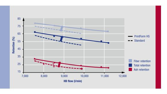
Compared to standard fabric: Higher retentions with PrintForm HS and 10-40% less retention aid dosage.
