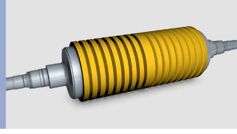
Web tension forces the lamellas of the WebTense roll cover to lie down and to the side - thus achieving the spreading effect.
