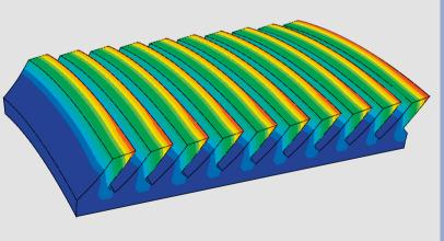
Deformation of the cover in radial direction.
