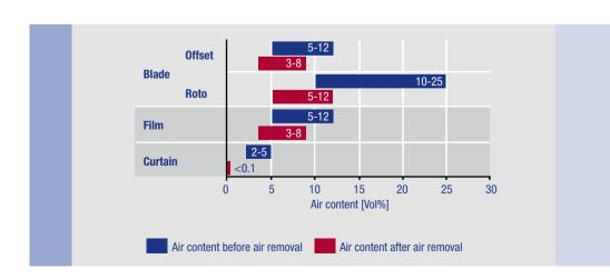
Fig. 1: Comparison of air contents before and after air removal for blade, film, and curtain processes.
