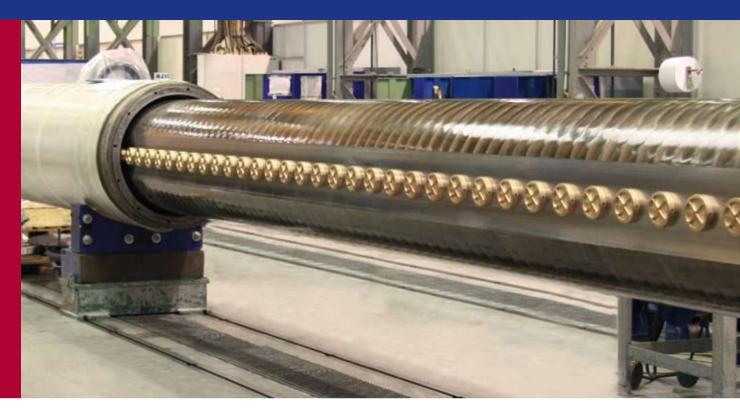
The same Nipcorect roll in the rebuild to counter support elements.
