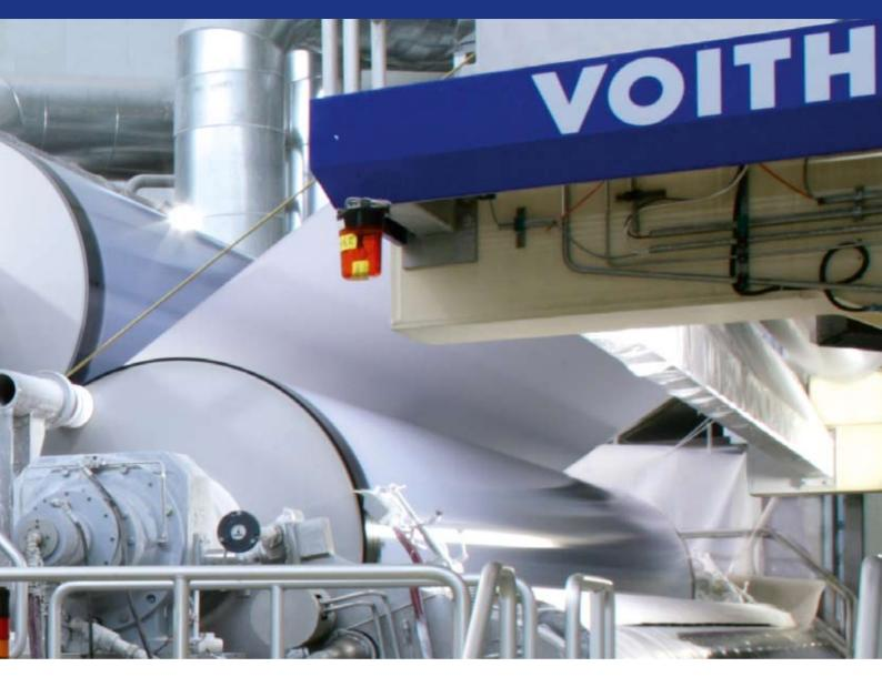
SpeedSizer film press with Luna roll covers provides a constant film coating process.
