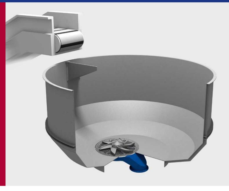
IntensaPulper IP-V with double break bottom tank and eccentric rotor.
