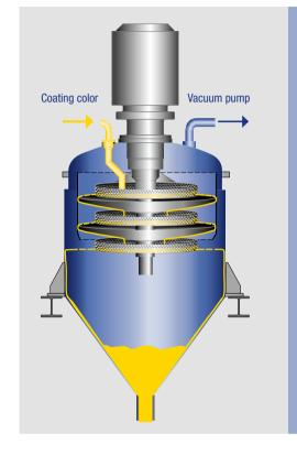
Fig. 2: The cascade principle of the AirEx AT-V provides for three times the surface.
