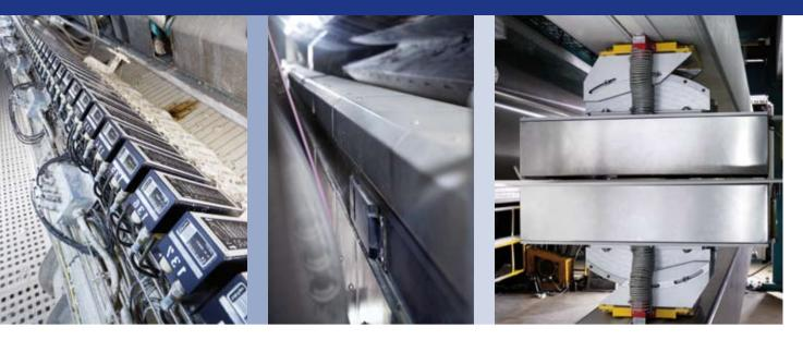
Continuous quality control system from the headbox to the reel: OnQ ModuleJet, OnQ EnviroScan and OnQ Scanner.
