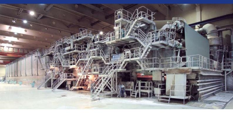
The PM 4 at UPM Steyrermühl was rebuilt to the modern DuoFormer CVB design.
