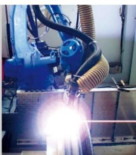
Welding robot for plasma welding.
