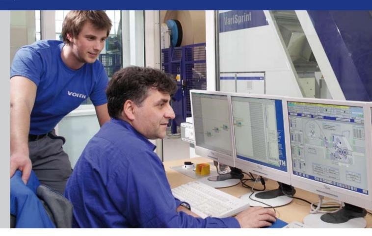
The virtual winder is a functional and graphic computer model which is connected with the real control system.
