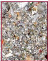
Left: Typical reject material from the heavy junk trap of a protector system.
