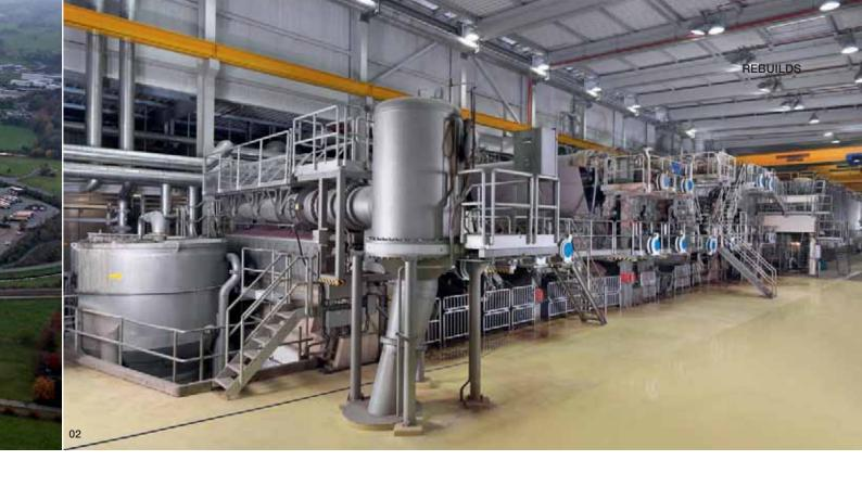
Fine screening in all lines was fitted with MultiFoil rotors and C bar Q screen baskets, and the centralized fiber aftertreatment was equipped with the latest generation of refining fillings. This has resulted in an exemplary overall solution that is both technologically sophisticated and economical. Line 1 has been in operation successfully since July 2011. Lines 2 and 3 started up in March and July of this year.
