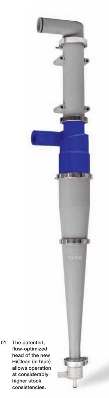
Poor Cinderella may have had to sort out the good from the bad by hand, but in a paper mill, this job is performed by the stock preparation unit, which removes impurities and recovers usable fibers. In the process, cleaning stages ensure quality in the low stock consistency range. HiClean, Voith Paper's new cleaner, is capable of processing substantially higher stock consistencies at the same level of efficiency.
