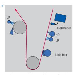
moisture profiling and increasing dryness can be located. The boxes are swiveled away during web threading.
