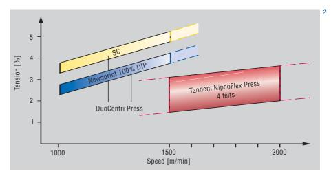
press sections need approx. 1.5% higher draw, *Fig. 2*. As further advantages of the closed draw configuration we expect less paper breaks, fast paper threading, no doctoring at center roll and high speed potential.
