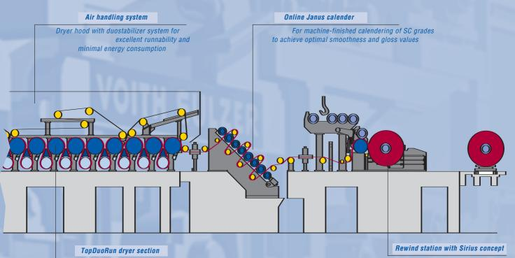
Reduced and more uniform shrinkage to improve paper quality Permanent support of paper web on dryer wire for optimal runnability and control Maximum possible reel diameter thanks to linear-load-controlled reeling for optimal roll structure and uniformity
