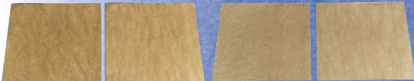
Pronounced stripes on kraftliner on a currently operating paper machine.
